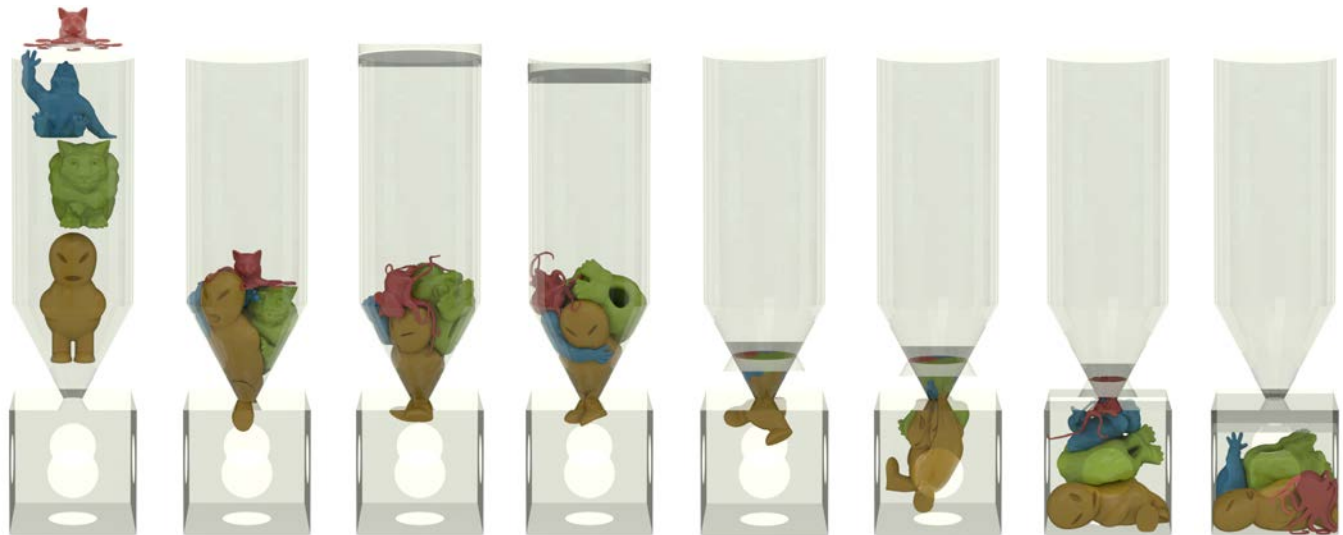
Fig. 1. Squeeze out: Incremental Potential Contact (IPC) enables high-rate time stepping, here with h = 0.01s , of extreme nonlinear elastodynamics with contact that is intersection- and inversion-free at all time steps, irrespective of the degree of compression and contact. Here a plate compresses and then forces a collection of complex soft elastic FE models (181K tetrahedra in total, with a neo-Hookean material) through a thin, codimensional obstacle tube. The models are then compressed entirely together forming a tight mush to fit through the gap and then once through they cleanly separate into a stable pile.
