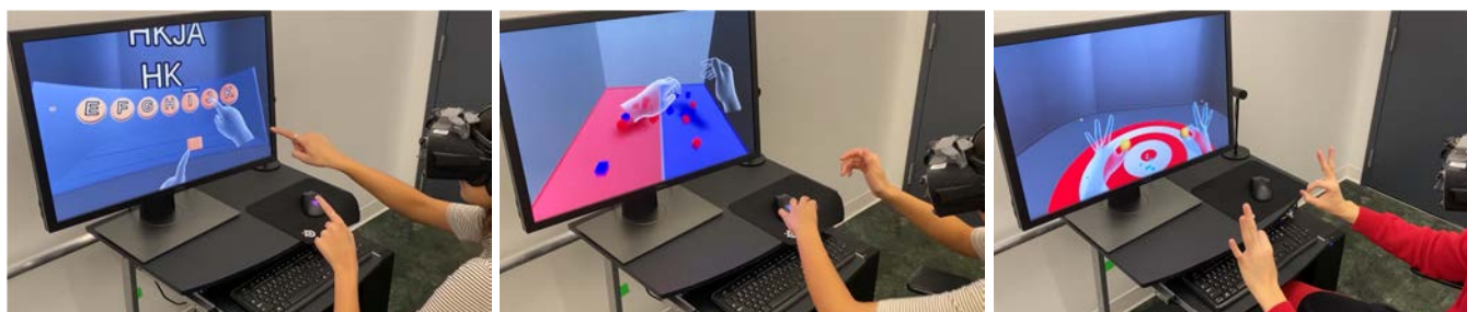
Fig. 1. We present a real-time hand-tracking system using four monochrome cameras mounted on a VR headset. We output the user's skeletal poses and rigged hand model meshes. Here we show some snapshots of users using our system to drive interactive VR experiences.
