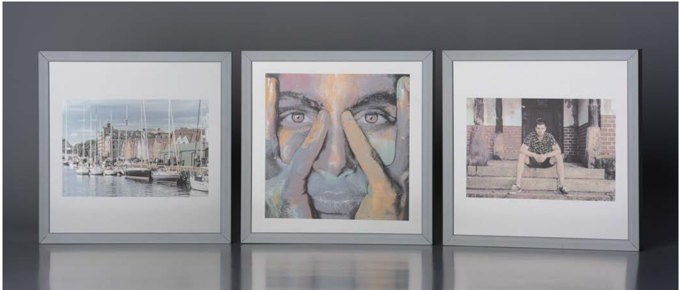
Fig. 1. Laser marked images on stainless steel using our proposed method (the plates are 13 \times 13 cm). Images © Piotr Didyk, Alexandr Ivanov, Sebastian Cucerca.
