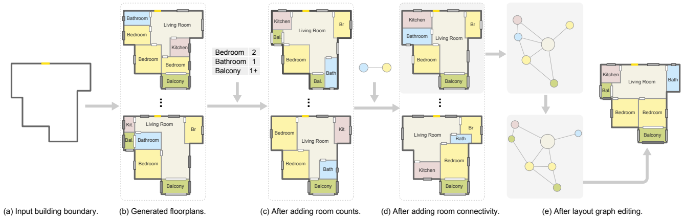
Fig. 1. Our deep neural network GRAPH2PLAN is a learning framework for automated floorplan generation from layout graphs. The trained network can generate floorplans based on an input building boundary only (a-b), like in previous works. In addition, we allow users to add a variety of constraints such as room counts (c), room connectivity (d), and other layout graph edits. Multiple generated floorplans which fulfill the input constraints are shown.
