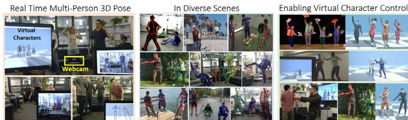
Fig. 1. Our real-time monocular RGB based 3D motion capture provides temporally coherent estimates of the full 3D pose of multiple people in the scene, handling occlusions and interactions in general scene settings, and localizing subjects relative to the camera. Our design allows the system to handle large groups of people in the scene with the run-time only minimally affected by the number of people in the scene. Our method yields full skeletal pose in terms of joint angles, which can readily be employed for live character animation. Some images courtesy [KNG Music 2019], [Music Express Magazine 2013a]. 3D characters from Mixamo [Adobe 2020].
