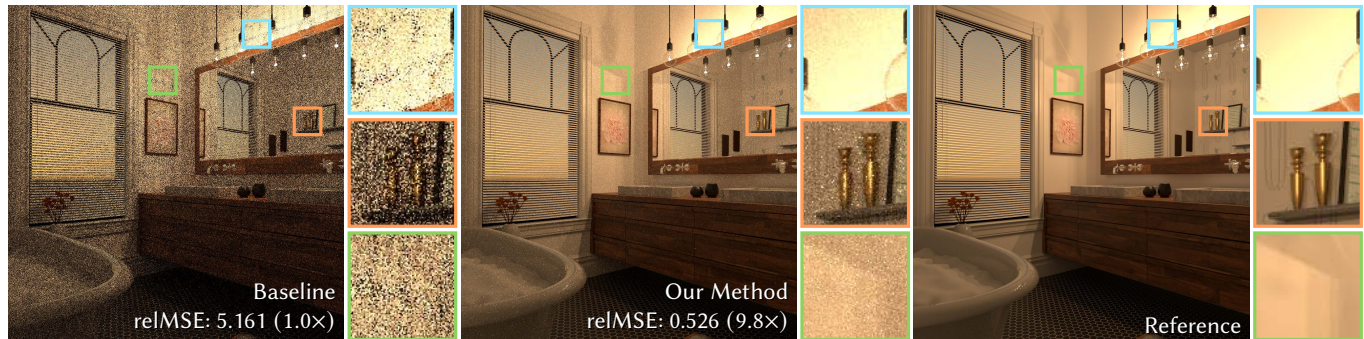
Fig. 1. BATHROOM scene rendered using our guided path tracer implementation with next-event estimation in 10 minutes each. The “baseline” (left) corresponds to a configuration similar to previous guiding approaches. “Our method” (middle) features significantly improved direction sampling in local path guiding by introducing a robust fitting procedure for parallax-aware mixtures, achieving a speedup of 9.8 in this scene.
