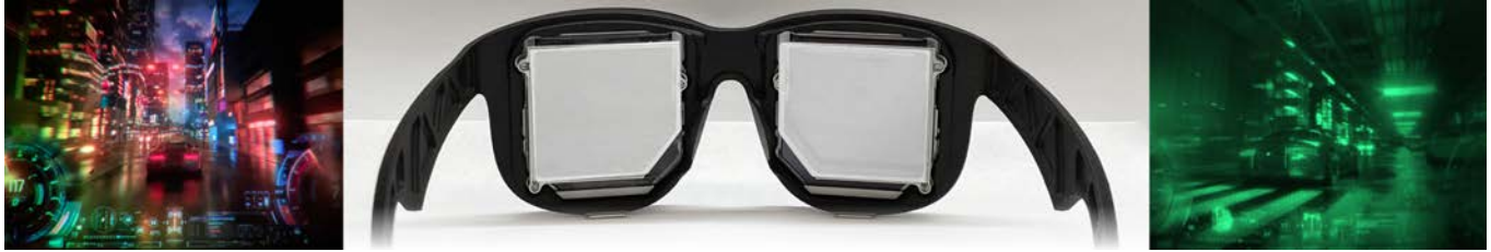
Fig. 1. Left: Photo of full color holographic display in benchtop form factor. Center: Prototype VR display in sunglasses-like form factor with display thickness of 8.9 mm. Driving electronics and light sources are external. Right: Photo of content displayed on prototype in center image. Car scenes by komba/Shutterstock.
