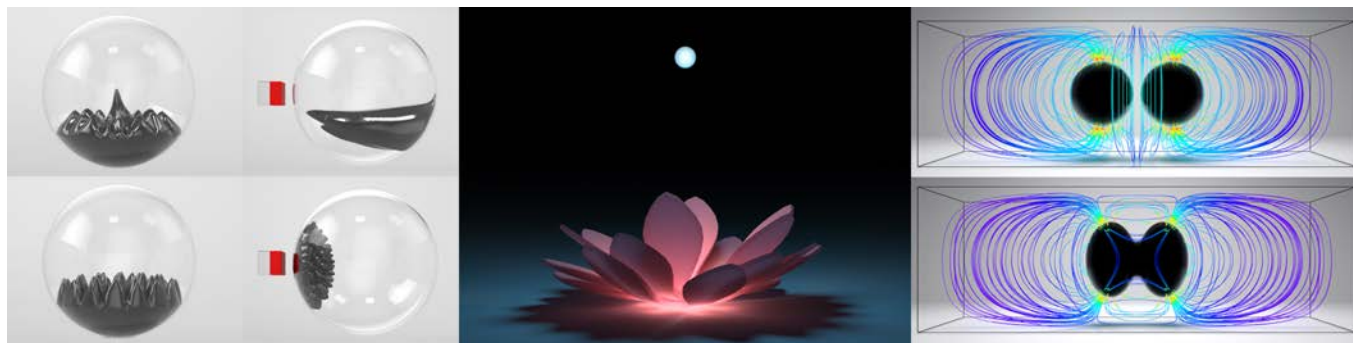
Fig. 1. Our unified level-set based approach can simulate and visualize the dynamics of a broad array of magnetic phenomena including ferrofluids, deformable magnetic bodies, rigid magnetic bodies, and multi-physics interactions.
