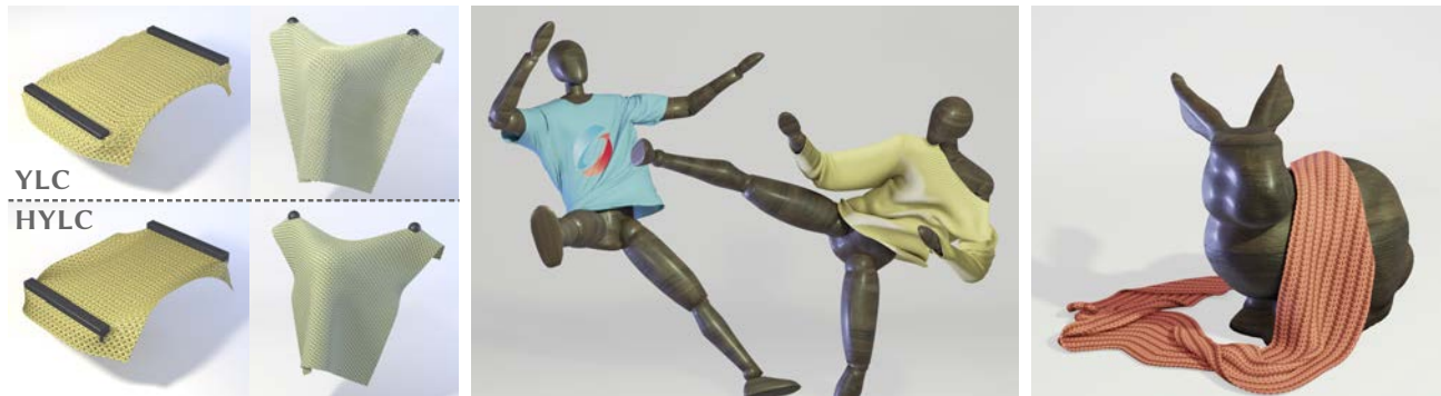
Fig. 1. Left: A comparison between direct yarn-level simulation (YLC) and simulation with our homogenized model (HYLC); our homogenized model accurately captures the non-trivial elastic stretching and bending response of the fabric. Middle and right: Results simulated with homogenized continuum models of woven and knitted patterns; our method allows us to efficiently compute large-scale simulations where direct yarn-level simulation would be prohibitively slow.
